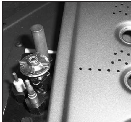
Figure 13. Ignitor assembly beside the burner.
